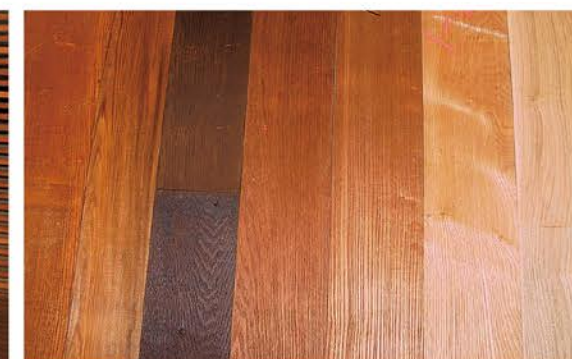
不同处理温度木材炭化颜色 The color of heat-treated wood at different treatment temperature
