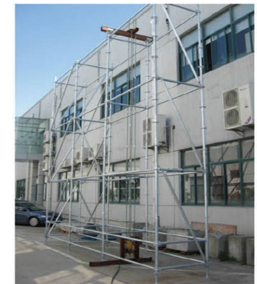
Ringlock Tower (One unit test)
