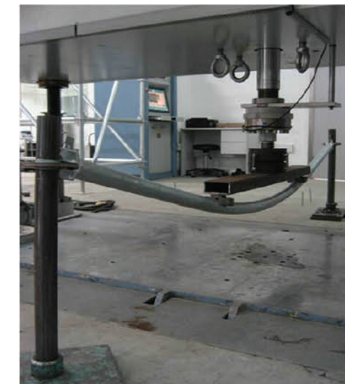
Ringlock Ledger (Load capacity test)
