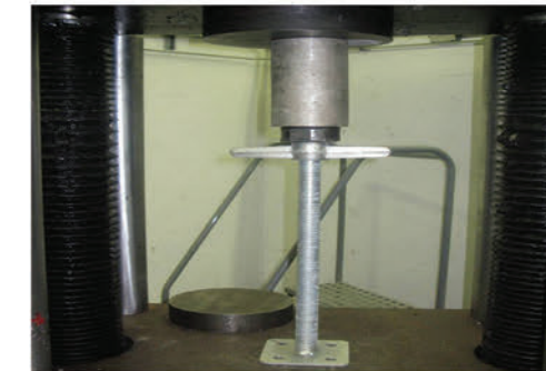
Base Jack (Test in different nut height)
