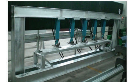
Steel Plank (Uniformly distributed load test)
