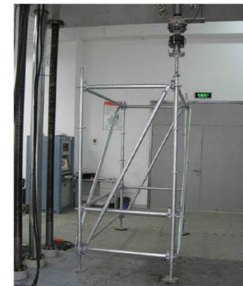
Ringlock Standard (Load capacity of single standard)
